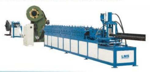
Decoiler → Leveling → Punching → Roll Forming → Cutting → Finished
