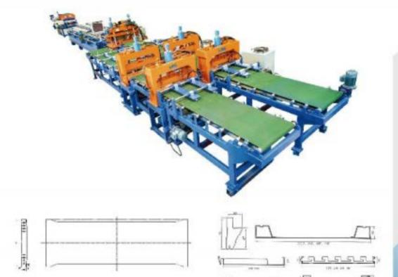
Decoiler → Leveling → Servo Feed & Punching → Roll Forming → Cutting → Conveyor 1# → Bending 1# → Conveyor 2# → Bending 2# → Conveyor 3#
