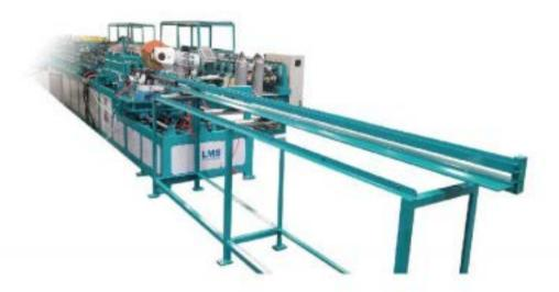
Decoiler → Leveling → Punching → Roll Forming → Welding (Step Beam) → Cutting → Finish
